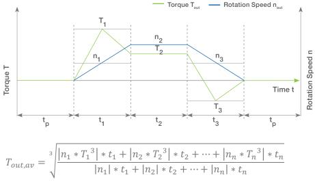
The calculated torque must be compared with the gear average  $T_{out,av} \leq T_A$ ? torque from the technical data sheet.
